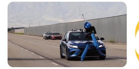
A dummy pedestrian struck by a vehicle during the test. Source: AAA
