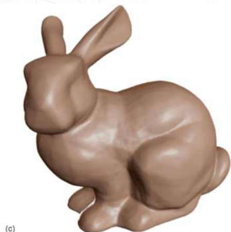
Fig. 3 - (a) depiction of the underlying implicit surface (b) 2D cross-section of the signed distance field, (c) rendered 3D surface recovered from \text{SDF} = 0 [9]
