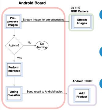
Generate image stream and process directly on Android board
