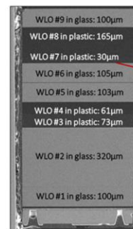
Camera – Cross-Section – SEM View ©2020 by System Plus Consulting
