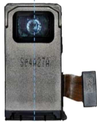
Front view of the camera module showing the position of the cross-sectional plane ©Yole SystemPlus 2024
